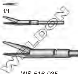
WS-516-035 1 x 5 mm Alligator Forceps Straight
